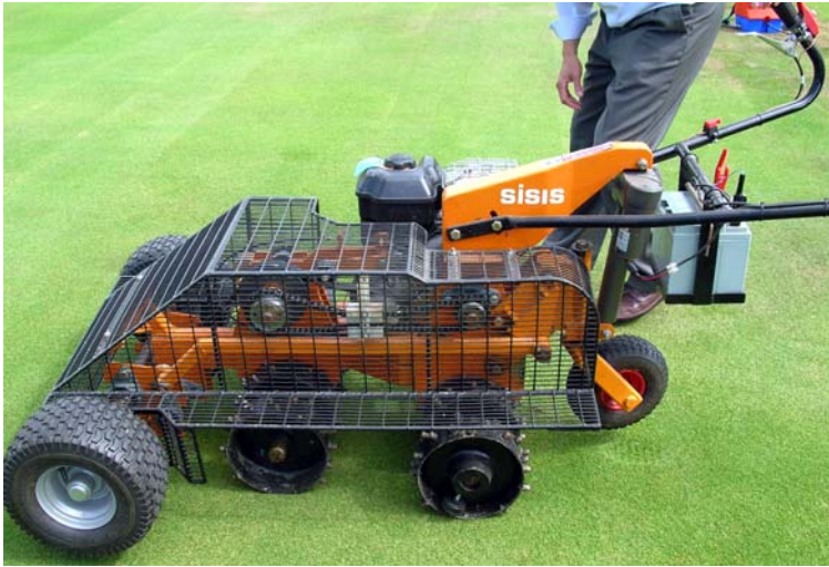
Figure 1. The SISIS wear machine, developed by The Sports Turf Research Institute (STRI) in England
